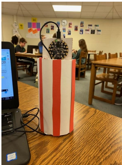
Mason Colburn Popcorn! When the popcorn container is tilted, the lights light up yellow and a popping sound starts to play.
